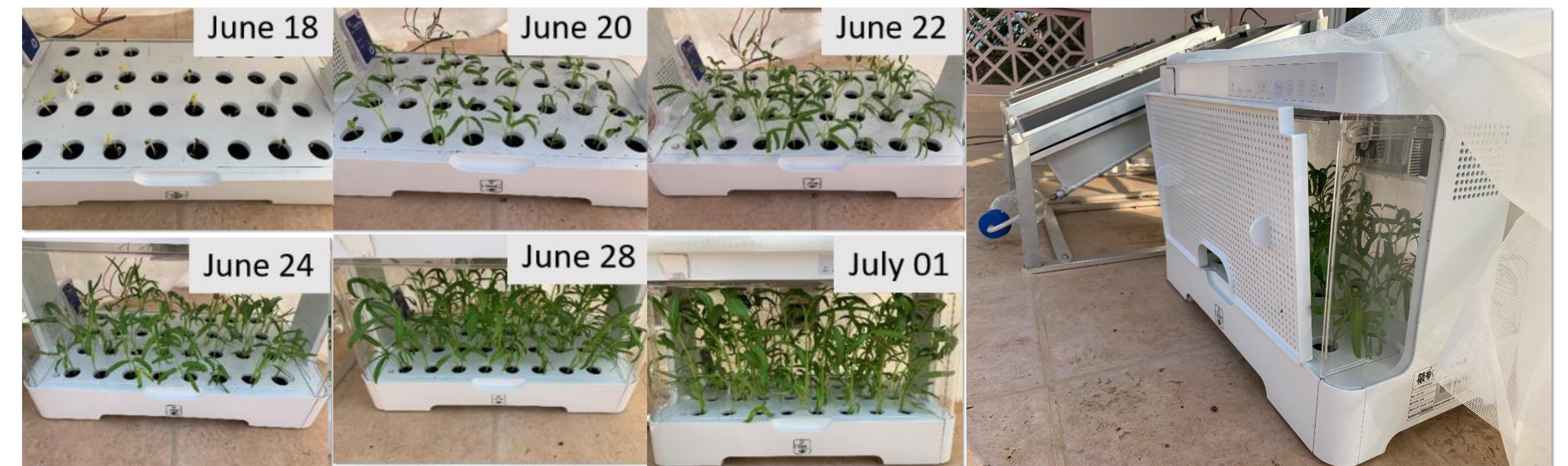
The growing status of water spinach in the outdoor field test and the bench-scale plant growing unit (PGU)
