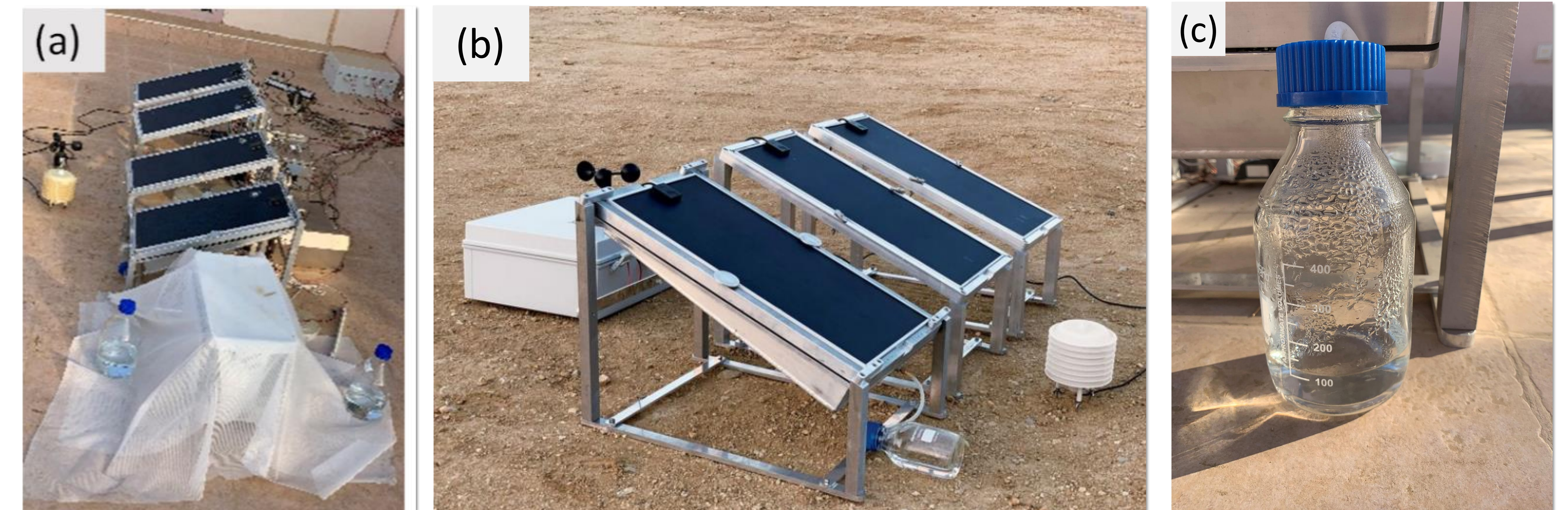
(a) Digital photo of WEC 2 P. (b) Digital photo of AWH water harvesting module. (c) Produced fresh water from one 0.6×0.3 m 2 prototype device
